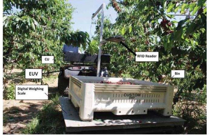
Figure 2. A variant of Labor Monitoring Device on an electric utility vehicle (EUV)
